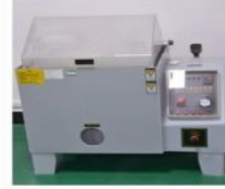
SALT SPRAY TESTER 盐雾测试仪
