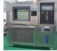
CONSTANT TEMPERATURE AND HUMIDITY MACHINE 恒温恒湿机
