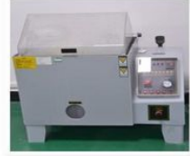
SALT SPRAY TESTER 盐雾测试仪
