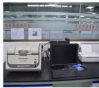
TIANRUI RoHS TESTER 天瑞ROHS检测仪
